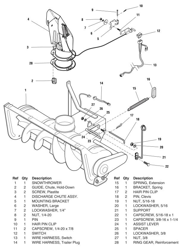
Figure 10. Initial Setup
